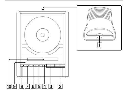
Display window 10 FUNCTION 7 (9, 16) OPEN/CLOSE ▲ 1 (9) Remote sensor 9 TUNER/BAND 6 (12) TUNING +/- 3 (12) VOL +/- 2
